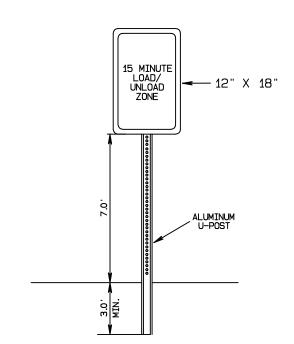
SIGN POST SHALL BE SO CONSTRUCTED AS TO HOLD SIGNS IN A PROPER AND PERMANENT POSISION, TO RESIST SWAYING IN THE WIND OR DISPLACEMENT BY VANDALISM.
